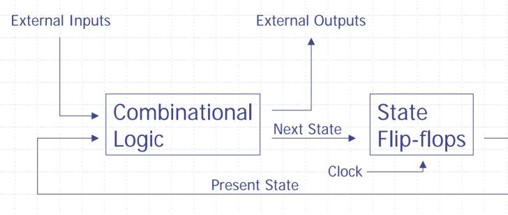
Maximum clock speed is determined by propagation delays in the Combinational Logic.
