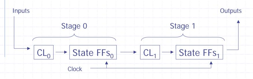
Propagation delays in  $CL_0$  and  $CL_1$  are less than delays in a single combined block of combinational logic, allowing for a faster clock speed.
