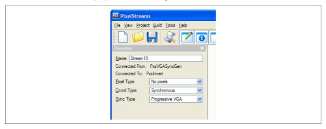
This window allows the user to set the name of the stream, and the type of data it will carry. The name entered will be the declaration name of the stream in the generated Handel-C code. The pixel type, coordinate type and the sync type of the data stream can also be set using the respective drop down boxes.
